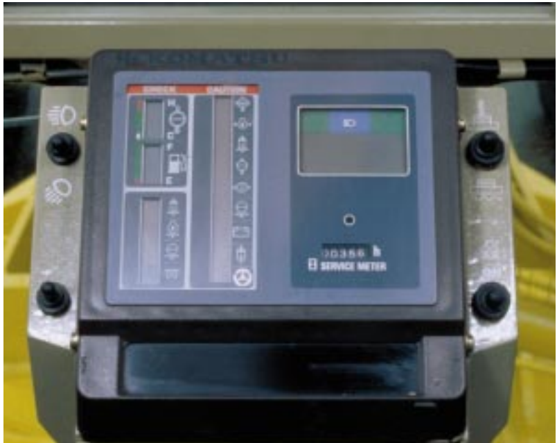
Electronic display and monitoring system continuously monitors all operating systems, keeping the operator well-informed of machine conditions.
