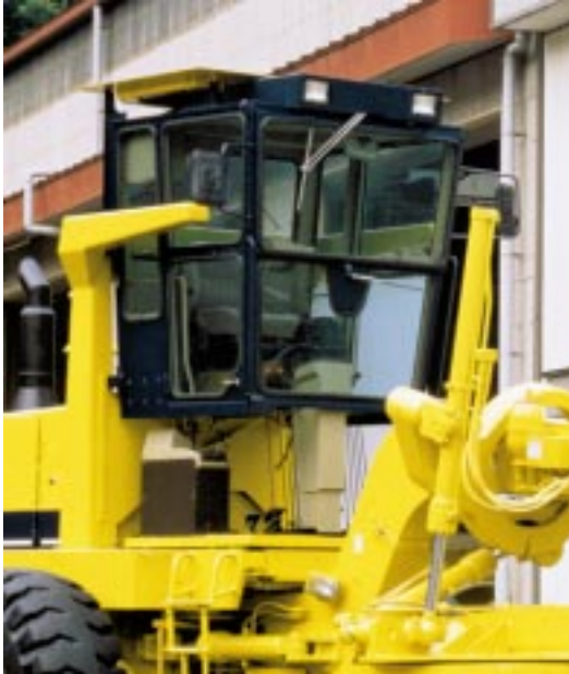
Elevating cab provides convenient accessibility for easy maintenance and repair functions.
