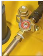
Fuel Drain Valve
