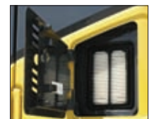
External air conditioner filter
