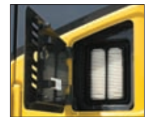
External air conditioner filter
